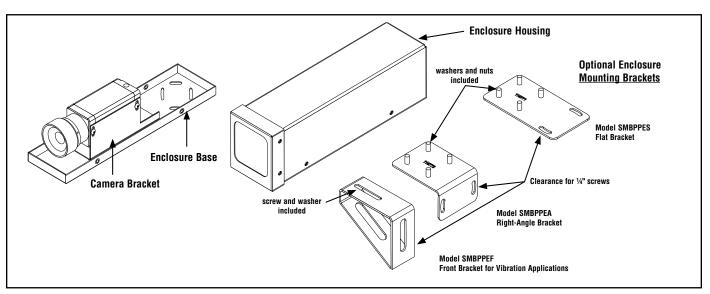
Figure 1. Assembling the enclosure
